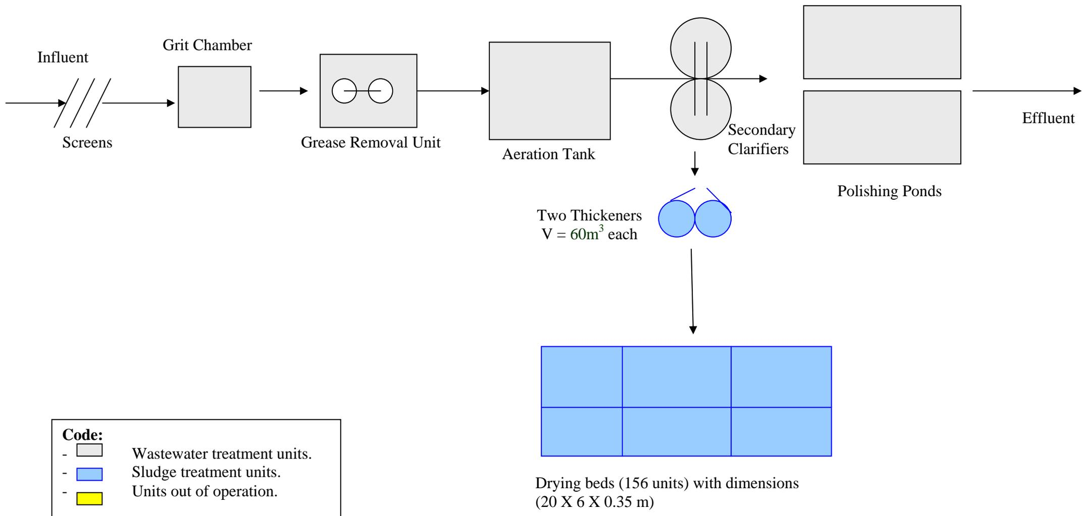
**Figure (1): Madaba Wastewater Treatment Plant / Schematic Flowchart.**
